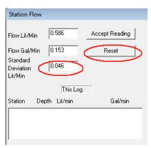
10. If the Standard Deviation is low and you are satisfied that the flow readings are stable, then click on Accept Reading.
