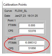
15. Enter the integrated FLOW\_SL cps number in the CPS section in point two of the FLOW\_SL calibration.
