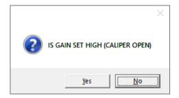
4. If you set the Gain to **HIGH**, you must click on **Open** on the **Caliper-Device** on the **Control Menu**. If you set the gain to **LOW**, you must click on **Close** on the **Caliper-Device** on the **Control Menu** (Even if already shown in Close position, you should press Close anyway).
