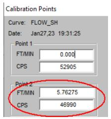
15. Enter the integrated FLOW\_SH cps number in the CPS section in point two of the FLOW\_SH calibration.
